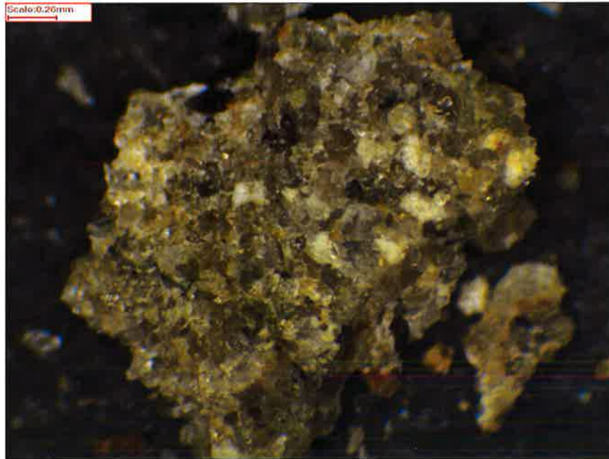
Figure 32 - Frontier Formation, Sample A05-1. A field micrograph shows an abundance of darker matter, indicating that this sample may contain too much lithic material for proppant.
