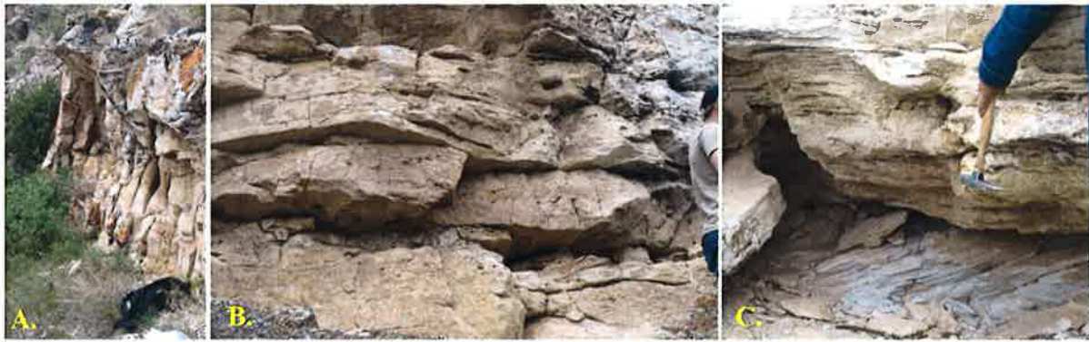
Figure 21 - Tensleep Formation: A] Lower dune sandstone, very fine grained where sample A07-1 was collected. B] Outcrop of reworked marine sandstone where sample A07-2 was collected. C] Contact between cross-bedded dune sandstone (A07-3 sample) and marine sandstone (A07-4 sample).
