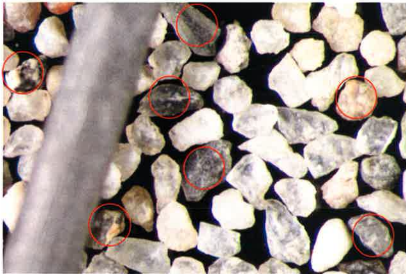
Figure 8 - Eolian glacial deposit near Ulm, MT (GFS-22). 70 mesh shown under a microscope with a 0.5mm pencil lead for scale. The red circles identify some of the lithic clasts that hinder the use of this eolian sand as proppant.
